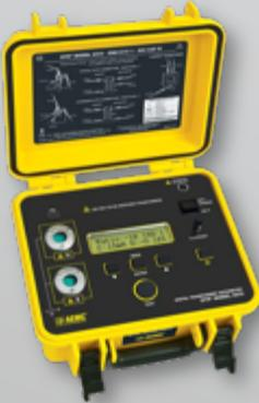
A yellow and black DTR 8510 AEMC single-phase TTR tester with a digital display and multiple test leads.            | <b>DTR 8510 AEMC</b>              |
