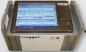
A portable, beige and grey MEGGER MWA 330 three-phase TTR tester with a color LCD screen and various control buttons. | <b>MEGGER MWA 330</b>             |
